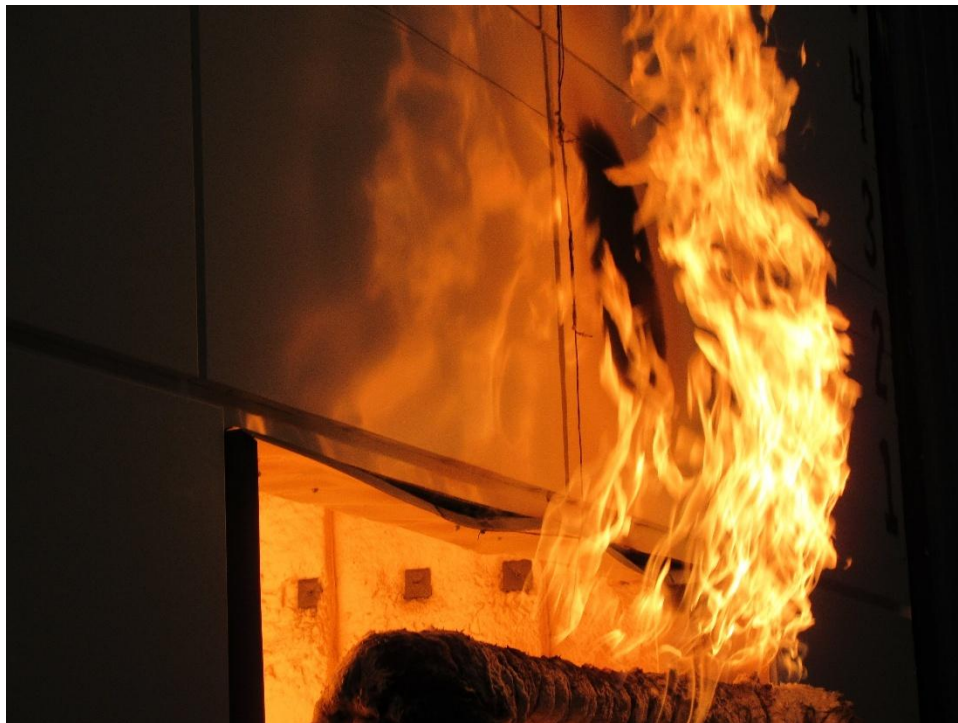
Photo No. 10 Discoloration of panels directly above window header – (11:46)
