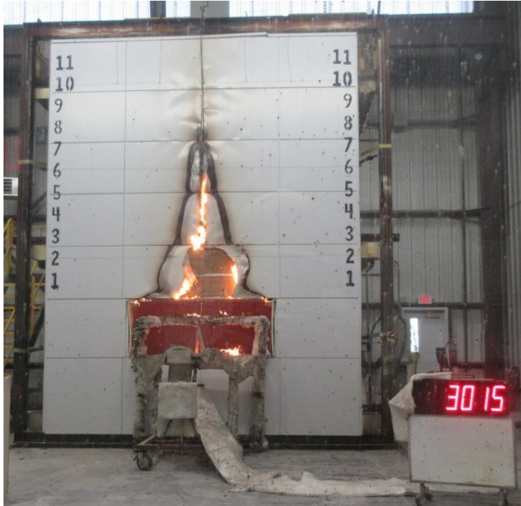
Photo No. 15 Wall assembly immediately following Test Conclusion
